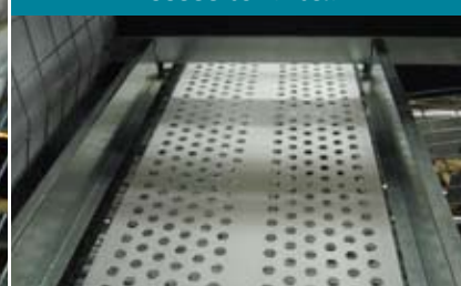
Strategically placed holes in nest belt keep belt clean, yet strong.
